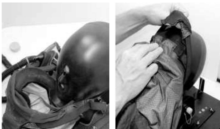
Figure 5-71. Placing the Mask on the IFSTHA
