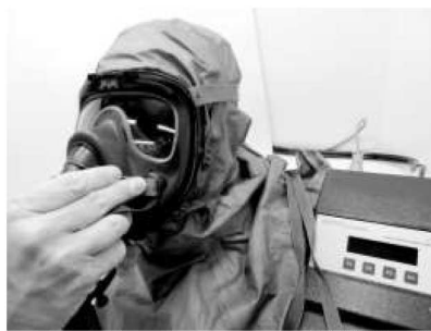
Figure 5-75. Attaching the Faceplate to the Hood Ring
