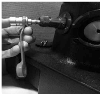
Figure 5-80. Plugging the M50 Drink/Fit Test Adapter In
