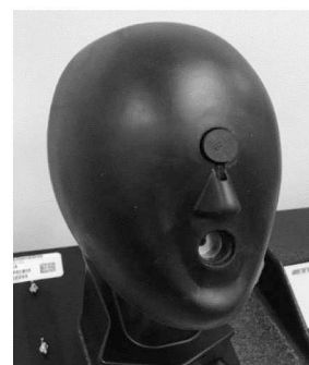
NO. 2 RUBBER STOPPER IN REAR HEADFORM PORT
