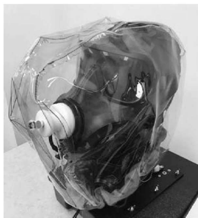
Figure 5-49. Placing the Mask Test Shroud Over the M53 Mask, Yellow Headform (Left) and IFSTHA (Right)
