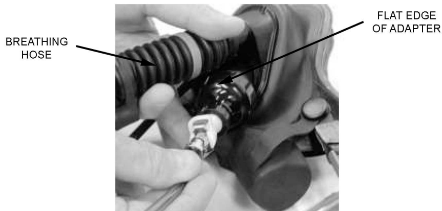
Figure 5-84. Attaching the MPU-5 Outlet Valve Plug/Adapter
