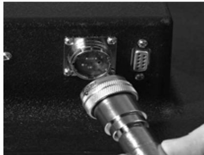
Figure 3-6. Power Interface Cable to Power Unit, Female End
