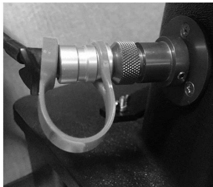
Figure 5-53. Seating the Spacer Ring on the Drink Tube
