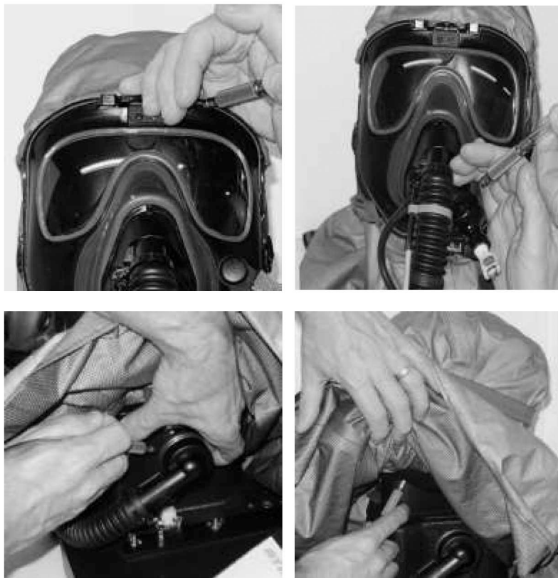
Figure 5-79. Examples of Probing the Mask (Clockwise From Top Left: Faceplate, Outlet Valve Assembly, Under the Hood, and Hose Port)
