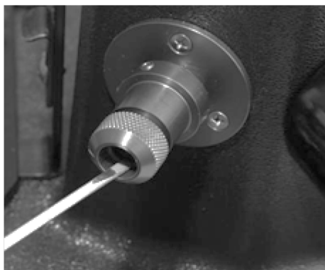
Figure 11-5. Replacement of the Drink Adapter O-ring
