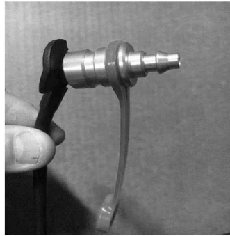
Figure 5-35. Attaching the M50 Drink/Fit Test Adapter
