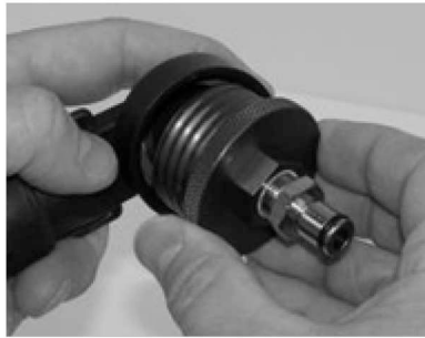
Figure 5-96. Attaching the Hose Test Adapter
