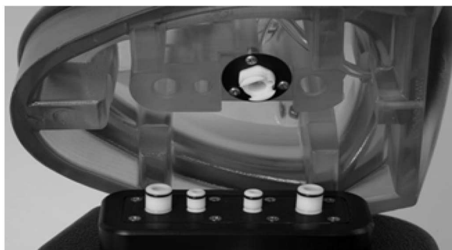
Figure 3-10. Headform and Pedestal Apart (Yellow Headform (Left) and Inflatable Face Seal Test Head Adapter (IFSTHA) (Right))
