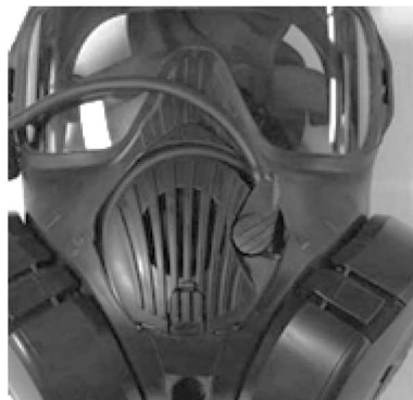
Figure 5-37. Turning the Drink Tube Lever to "OPEN" Position
