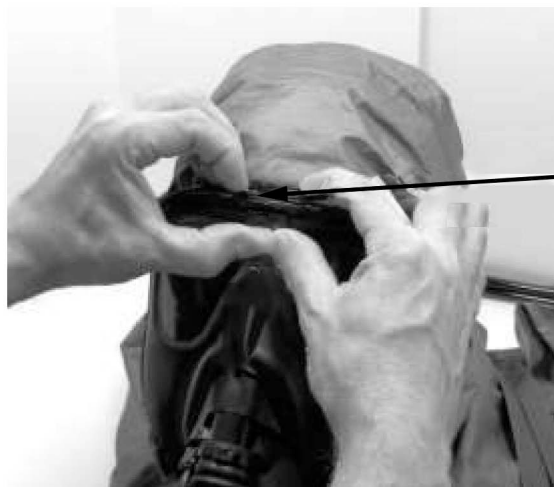
Figure 5-76. Double Checking the Faceplate Connection
