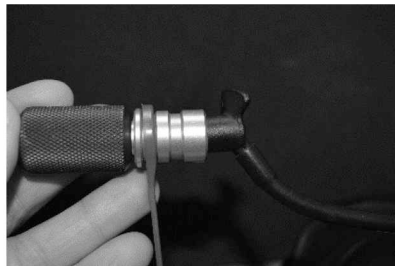
Figure 5-36. Plugging Into the Fit Test Sampling Adapter
