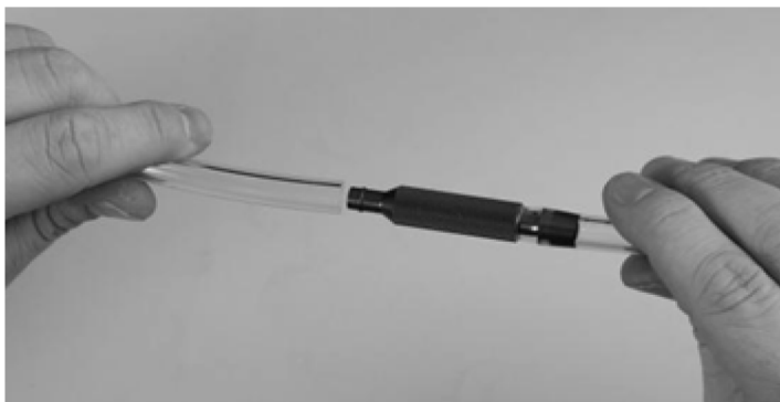
Figure 3-15. Y-Hose Aerosol Extension Connecting to Aerosol Probe Hose
