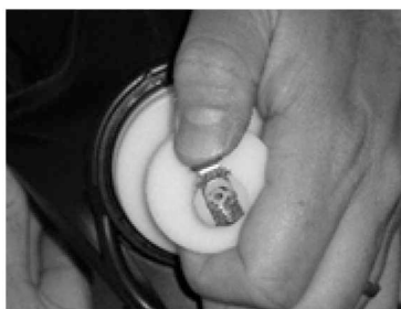
Figure 5-48. Attaching the M53 Outlet Valve Plug/Adapter
