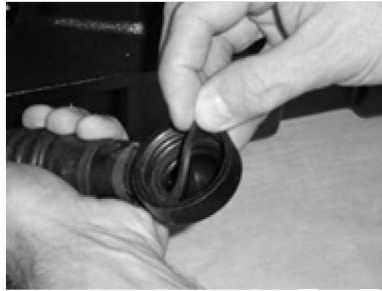
Figure 5-95. Gasket in Canister End of Hose
