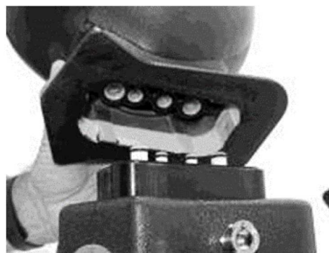
Figure 3-10. Headform and Pedestal Apart (Yellow Headform (Left) and Inflatable Face Seal Test Head Adapter (IFSTHA) (Right))
