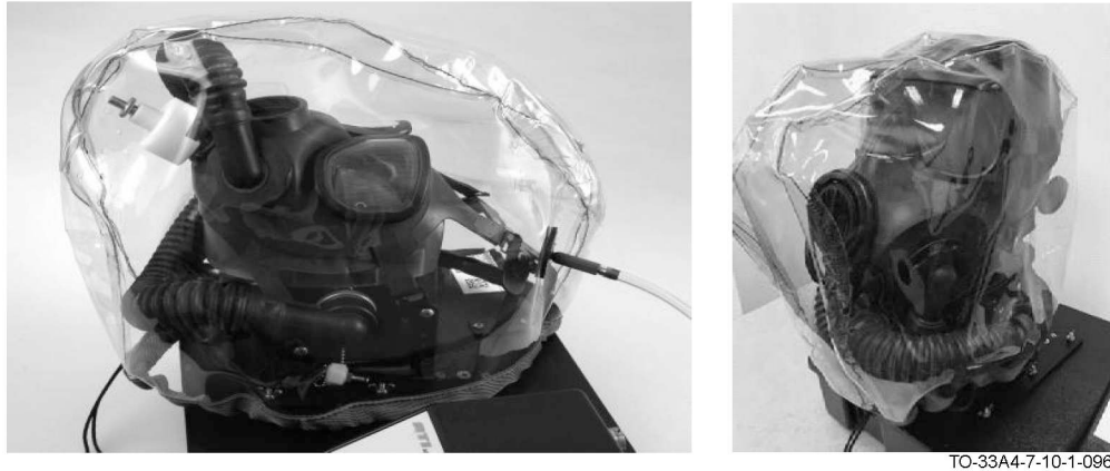
Figure 5-89. Test Shroud Over Mask with Hose, Yellow Headform (Left) and IFSTHA (Right)
