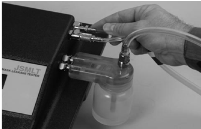
Figure 3-16. Fit Test Interface Tubing Assembly
