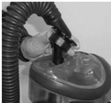
Figure 5-100. Plugging the M40 Series Hose Connector Into the Vacuum Port
