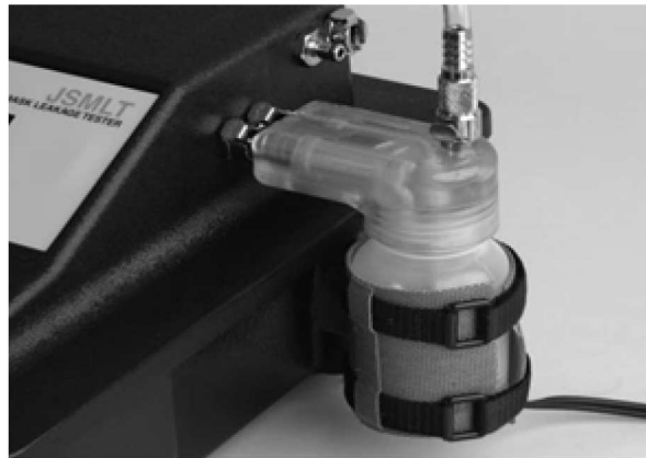
Figure 3-18. Oil Warmer Attached
