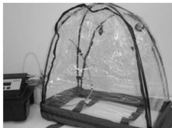
Figure 8-1. Fit Test Aerosol Setup
