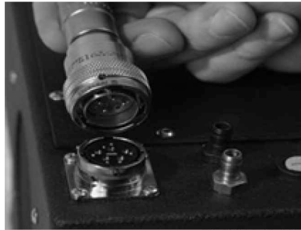
Figure 3-5. Power Interface Cable to Power Unit, Male End
