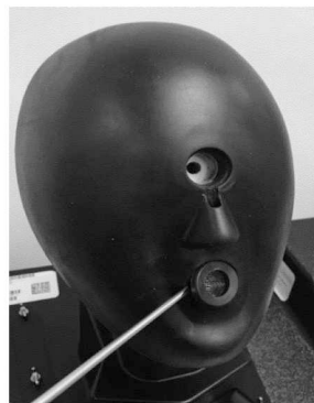
Figure 5-27. Lint Screen, Yellow Headform (Left) and IFSTHA (Right)
