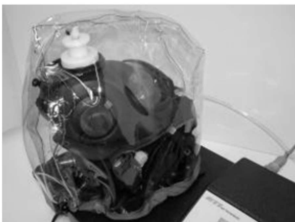
Figure 5-49. Placing the Mask Test Shroud Over the M53 Mask, Yellow Headform (Left) and IFSTHA (Right)
