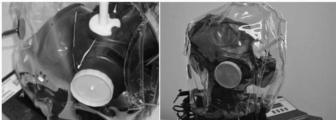
Figure 5-29. Mask Test Shroud Over M50/51 Using Yellow Headform (Left) and IFSTHA (Right)
