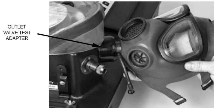
Figure 7-1. Outlet Valve Test [VALVE]
