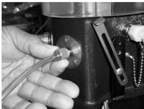
Figure 5-44. Installing the M50 Outlet Valve Hose
