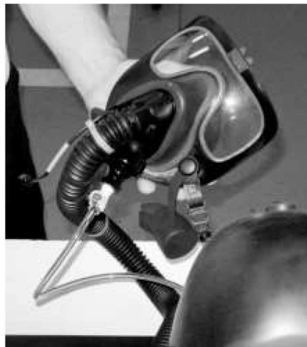
Figure 5-85. Supporting the Mask During the Outlet Valve Test [VALVE]
