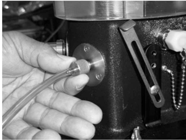
Figure 5-18. Connection of the M50 Outlet Valve Hose
