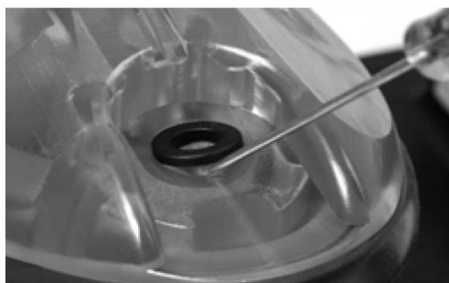
Figure 5-92. Removal of the Lint Screen, Yellow Headform (Left) and IFSTHA (Right)
