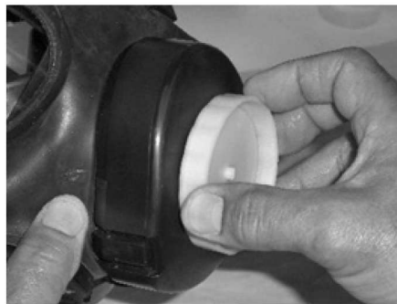
Figure 5-24. Attachment of the M50 Filter Plug
