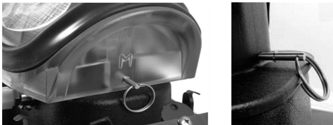
Figure 3-11. Headform and Pedestal Assembled (Yellow Headform (Left) and IFSTHA (Right))
