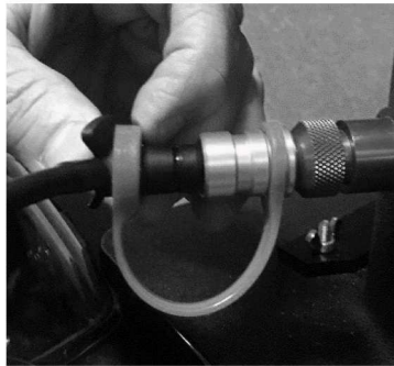
Figure 5-52. Attaching the Spacer Ring
