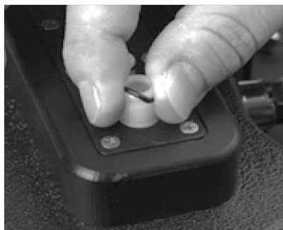
Figure 11-6. Replacement of the External O-ring
