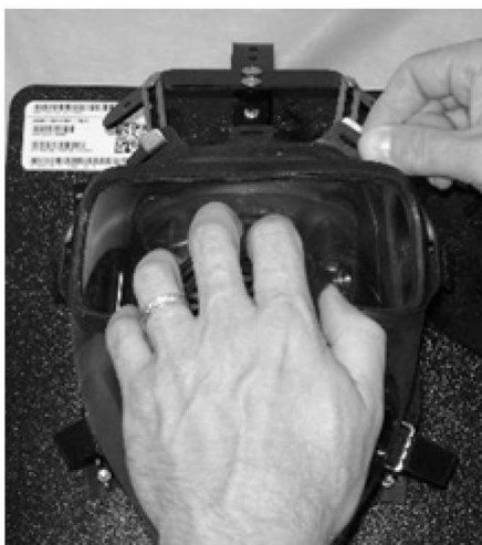
Figure 5-47. Compressing the Nosecup
