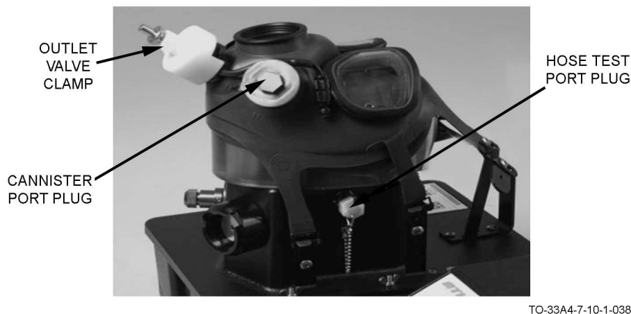
Figure 5-5. Mask with Adapters
