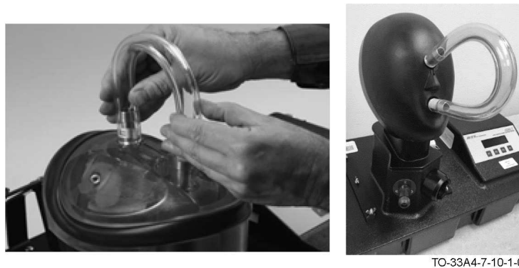
Figure 11-9. Inserting the Mask Passing Tube, Yellow Headform (Left) and IFSTHA (Right)
