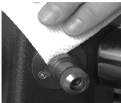
Figure 11-7. Cleaning the Drink Tube Adapter
