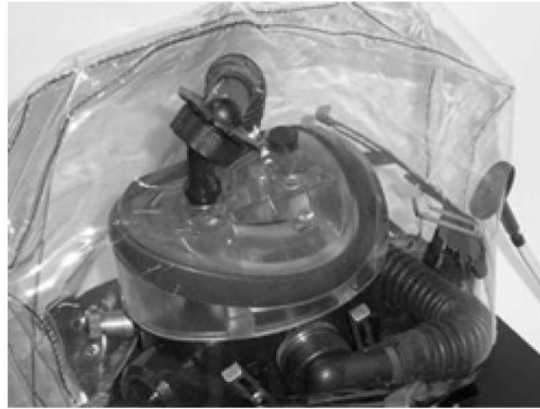
Figure 5-101. Placing the Mask Test Shroud Over the Test Head Hose
