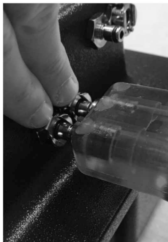
Figure 3-4. Attaching the Aerosol Generator Assembly to CU Into Generator Ports
