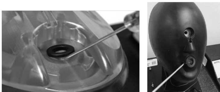
Figure 11-8. Removal of the Lint Screen, Yellow Headform (Left) and IFSTHA (Right)
