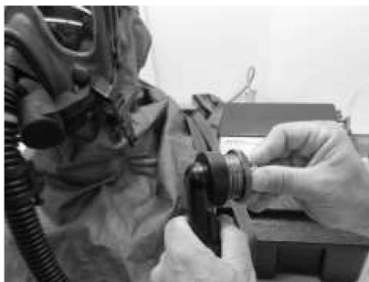
Figure 5-64. Attaching the Hose Test Adapter
