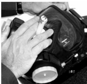
Figure 5-28. Compressing the Nosecup
