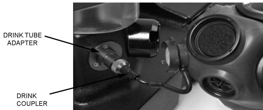
Figure 6-1. Drink Tube Flow Test Setup
