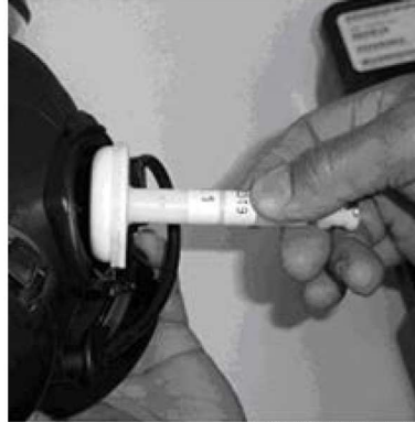
Figure 5-25. Installing the M50 Outlet Valve Plug/Adapter
