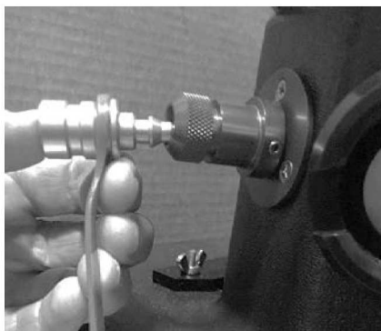
Figure 5-30. Attaching the M50 Drink/Fit Test Adapter
