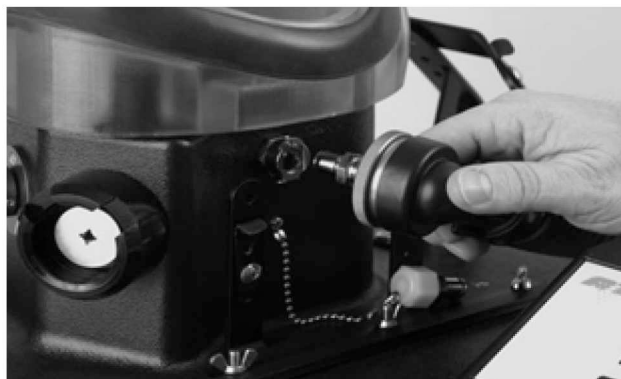
Figure 5-88. Attaching the Mask Hose Test Adapter
