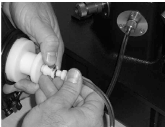
Figure 5-54. Installing the M50 Outlet Valve Hose
