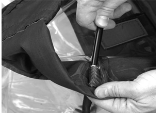
Figure 3-12. Fit Test Support Rod Into Nylon Corner Pouch
