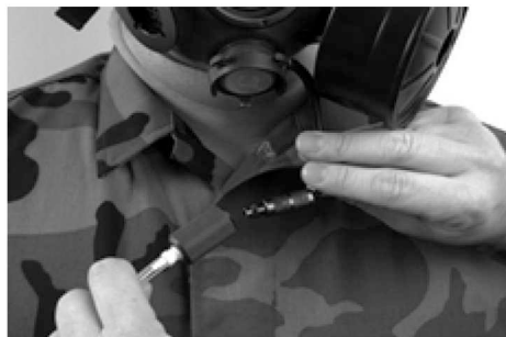
Figure 8-2. Attaching the Fit Sampling Adapter
